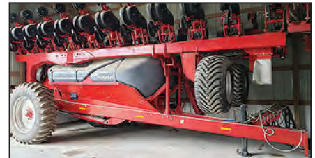
Horsch 24 row 30 inch compplanter, 2x2 fertilizer, 1000 gallon tank, hydraulic down pressure, electric drive meters, 130 bushel seed tank, iso buss plug and play monitor, showroom condition, $195,000
