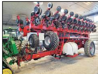
Horsch 2430 Maestro corn planter, 2017 model, new in 2019, 12,000 acres, in-furrow fertilizer, Sunco 2x2x2 fertilizer openers, 18.4x42 tires, 1400 gallon fertilizer tanks, plug and play isobus. $179,000
