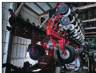
2023 Horsch Maestro SP2430, 24row 30in, 6500ac, Precision Planting Vsets, Speed Tube, Delta Force, Furrow Force, Gen 3 20/20, 25in tracks 2x2x2 fertilizer with 750gal tank plus 800 gal saddle tanks. $359,000
